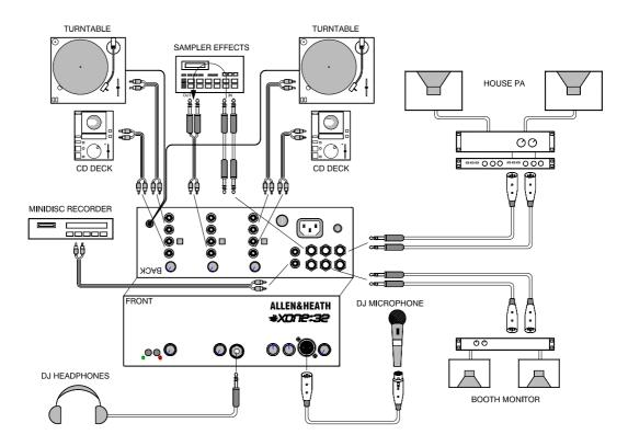
**DJ Microphone and Headphones**: The DJ plugs the preferred headphones and microphone (if required) into the front of the console. It is not uncommon for several DJ's to perform their sets during a session plugging in their own mic and headphones each time. The console cue system works with the headphones to let the DJ cue tracks and preview the mix before going live.
