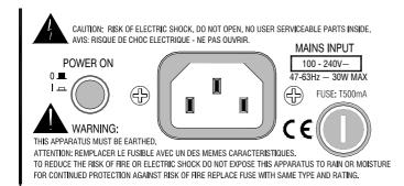
**Connecting Mains Power** Read the SAFETY INSTRUCTIONS printed at the front of this User Guide and on the rear panel. Check that the correct mains lead with moulded plug has been supplied with your console. The power supply accepts 50/60Hz AC mains voltages within the range 100-240V without changing any fuses or settings.
