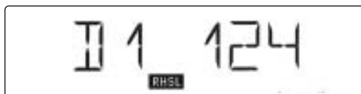
Example 1: Dropout no. 1 occurred after 124 seconds.
