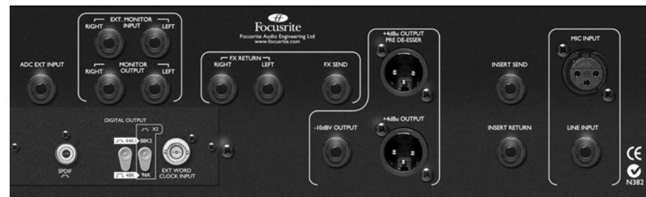
The VoiceMaster Pro features MIC INPUT XLR and LINE INPUT TRS connectors on the rear panel, with the MIC INPUT duplicated on the front fascia together with a
