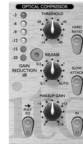
**IN (switch)** – Switches the OPTICAL COMPRESSOR into the signal path. When engaged, the red LED in the switch cap is lit.
