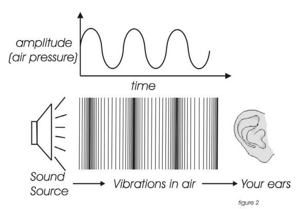
**Frequency**– The rate of vibration in sound measured in Hertz (Hz or cycles/second) (figure 3). Our ears can hear from 20 to 20,000 Hz. Frequency corresponds to the musical term, pitch. A low frequency corresponds to a low-pitched sound such as a bass; a high frequency sound corresponds to a high pitched sound such as a piccolo. In music, a change in pitch of one octave higher equals a doubling of the frequency.
