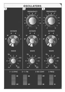
The Oscillators are the main sound source of the Voyager. The oscillators in the Voyager are all analog Voltage Controlled Oscillators, or VCOs. They feature a temperature regulation circuit that provides them with excellent tuning stability. The VCOs can produce a total musical range of 8 ½ octaves! In addition, the frequency of oscillator 3 can be set to sub-audio (<20Hz) vibrations for use as a second LFO.
