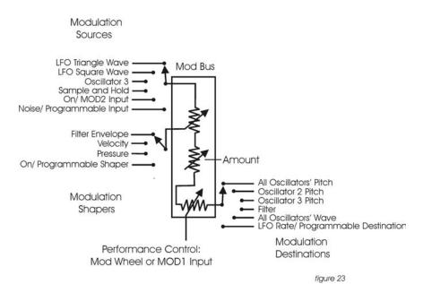
Here's a block diagram of a Mod bus (figure 23):
