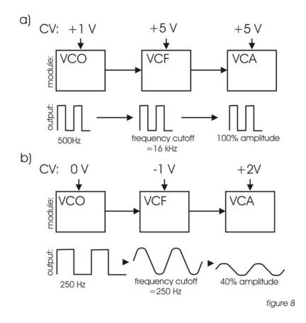
**Modulation** - Modulation is the use of a CV to affect a voltage-controlled circuit. Modulation has a source, destination, and amount. This could be as simple as the filter cutoff of a VCF (a modulation destination) being changed by the front panel cutoff control (the source), or as complex as mixing multiple CVs together to modulate filter cutoff. Modulation is used in synthesis to create complex sounds and add variation.
