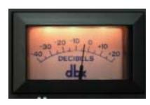
When set to Input, the VU Meter indicates the plug-in input level in dB. When set to Output, the VU Meter indicates the plug-in output level in dB. When set to Gain Change, the VU Meter indicates the amount of Gain Reduction in dB.
