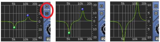
Figure 8. Vertical resolution of the Response Curve can be changed with the Zoom buttons
