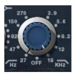
The independent low and high cut filters are controlled by the dual-concentric knobs to the right of the low band (see Figure 67 on page 225). The controls specify the fixed frequency of the cut filter. The cut filters have an 18 dB per octave slope.
