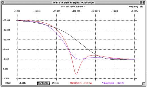
Figure 59. Effect of Bandwidth control on response curve in Shelf mode
