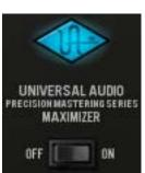
The Power switch determines whether the plug-in is active. This is useful for comparing the processed settings to the original signal or bypassing the plug-in to reduce the UAD DSP load (load is not reduced if *UAD-2 DSP Load-Lock* is enabled).
