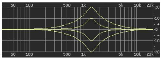
Figure 11. Parametric Type I response
