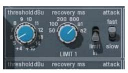
Controls in this section only function when the limiter is enabled with the "limit In" switch (the Power switch must also be on).
