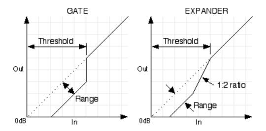
Figure 76. The Neve 88RS Gate/Expander diagram
