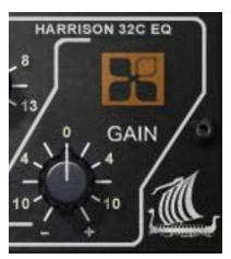
The Gain knob controls the signal level that is output from the plug-in. The default value is 0 dB. The available range is ±10 dB.
