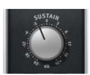
Sustain enables amplification or attenuation of the sustain of a signal by up to ±24 dB.
