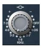
The midrange band is controlled by dual-concentric knobs, delivering smooth semi-parametric midrange equalization.
