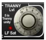
This control determines the amount of Tranny processing (see "The Tranny Processor" on page 102 for a detailed description). Higher values make the Tranny effect more prominent. Increasing the Tranny level also increases the signal THD (see "THD Indicators" on page 105), and the sensitivity of the Warmth processor (page 106). A value of 5 is the unity setting.
