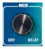
This continuous control adjusts the blend between the original dry signal and the processed wet signal(s). The available range is 0 – 100%.
