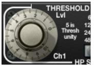
This knob enables manual threshold control of the FATSO compressor. Higher values lower the threshold, and therefore increase the amount of compression. A value of 5 is the unity setting.
