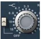
The high band delivers smooth high frequency shelving or peak equalization. The inner knob controls the band gain, and the outer ring selects the frequency or band disable.
