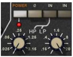
In addition to the four-band EQ, the Harrison 32C offers two cut filters, one each for low and high frequencies. The slope of the cut filters is 12 dB per octave.
