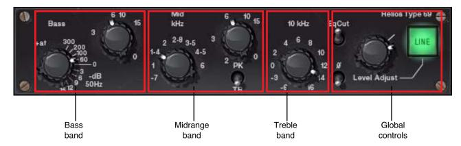
Figure 48. Helios 69 band control layout
