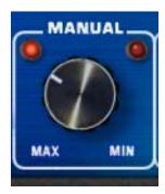
This continuous control determines the delay time of the processor. The delay time is modulated by the Sweep LFO when the Width value is higher than 0%.
