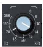
The independent low and high cut filters are controlled by the dual-concentric knobs to the right of the low band. The controls specify the fixed frequency of each cut filter.
