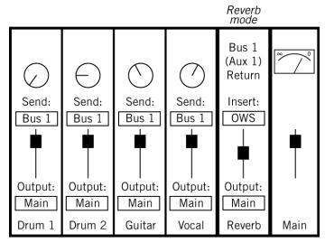
Figure 83. DAW signal routing in Reverb mode using a traditional effect send/return configuration.
