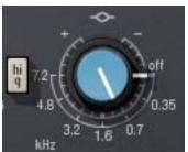
The midrange band is controlled by dual-concentric knobs, delivering smooth semi-parametric midrange equalization with a choice of two bandwidths. The inner knob controls the band gain, and the outer ring selects the frequency or band disable.
