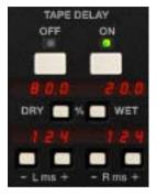
These parameters control the built-in Tape Delay, which creates tape echo effects. For an overview of this feature, see "Tape Delay" on page 22. The Tape Delay controls are not available in the original hardware.
