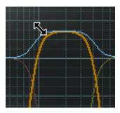
If the cursor is moved to the upper-left region of the three center bands (LMF, MF, HMF), the gain and bandwidth can be adjusted simultaneously, without changing the center frequency. In this case the cursor changes to a diagonal arrow when hovered over the hot spot to indicate the direction available for dragging.
