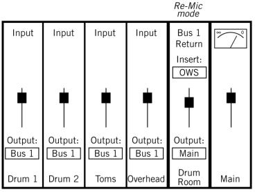
Figure 84. DAW signal routing with OWS in Re-Mic mode on a drum submix
