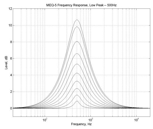
Figure 108. Pultec MEQ-5 Low Peak Response
