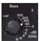
The Bass knob has a dual purpose. It specifies the amount of attenuation when the low band is in shelving mode, and specifies the frequency of the low frequency peak filter when the Bass Gain knob is not zero.
