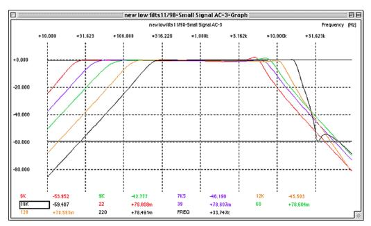
Figure 60. High Pass and Low Pass filter response curves (standard version)
