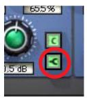
Each band can be switched from parametric mode to shelf mode by clicking the shelf enable button. The button is off by default. To enable shelving on any band, click the shelf button.
