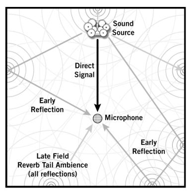
Figure 81. The main signal components in an acoustically recorded sound
