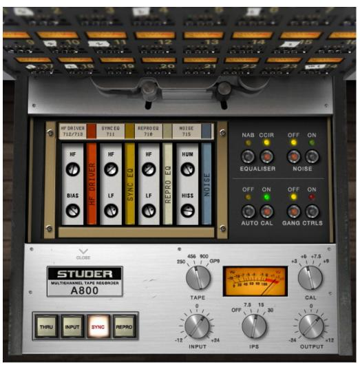
Figure 134. The Studer A800 plug-in window with exposed secondary controls
