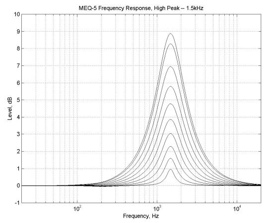
Figure 110. Pultec MEQ-5 High Peak Response
