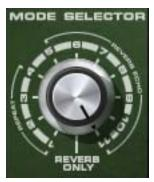
The RE-201 is a combination of a tape echo and a spring reverb effect. Echo, reverb, or both can be selected with the Mode Selector to determine which effect(s) are active.
