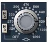
The low-midrange band delivers smooth low-mid frequency peak equalization with a choice of two bandwidths. The inner knob controls the band gain, and the outer ring selects the frequency or band disable.
