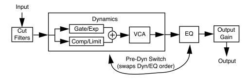
Figure 75. Simplified signal flow within UAD Neve 88RS
