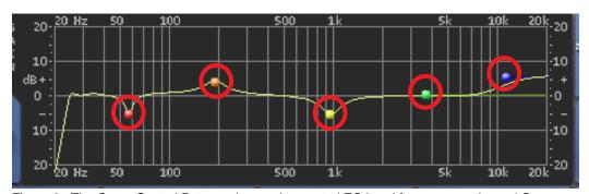
Figure 9. The Curve Control Bats can be used to control EQ band frequency, gain, and Q
