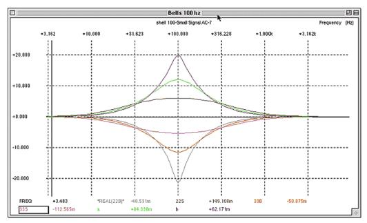
Figure 58. Effect of Bandwidth control on response curve in Bell mode
