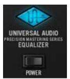
The Power Switch determines whether the plug-in is active. This is useful for comparing the processed settings to the original signal, or to bypass the plug-in to reduce the UAD DSP load (load is not reduced if *UAD-2 DSP LoadLock* is enabled).
