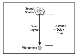
Figure 82. Illustration of Distance Delay. When set to aligned, this "extra" time is eliminated.
