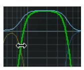
If the cursor is moved to where two bands crossover, the crossover frequencies can be adjusted, without changing the gain or center frequency. In this case the cursor changes to a left/right arrow when hovered over the hot spot to indicate the direction available for dragging.
