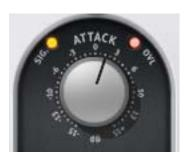
Attack enables amplification or attenuation of the attack of a signal by up to  $\pm 15$  dB.
