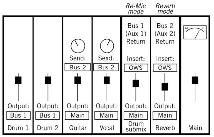
Figure 85. DAW signal routing in a workflow with two Ocean Way Studios plug-in instances. One uses Re-Mic mode for the drum submix, and the other uses Reverb mode for the guitar and vocals.
