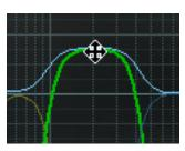
If the cursor is moved slightly lower than the above example, the gain and center frequency can be adjusted simultaneously, without adjusting the bandwidth. In this case the cursor changes to an up/down/left/right arrow when hovered over the hot spot to indicate the direction available for dragging.
