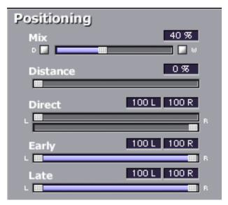
Figure 117. RealVerb Pro Positioning panel
