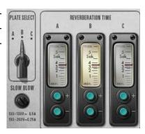
The original damper controls are remote control devices, usually found somewhere near the control room for quick access. Our hybrid panel combines three remotes into the panel, with a switch to select each of the three available systems.
