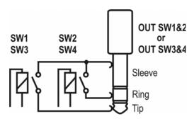
SWITCH outputs are galvanically separated to avoid grand loops. It is recommended to use the connectors with plastic jackets to avoid occidental connection with signal grand.
