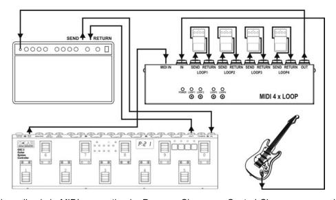
The control is realized via MIDI connection by Program Change or Control Change commands. It enables to choose the way of controlling either by recalling the program setting the loops state or by Control Change commands (switching of individual loops).
