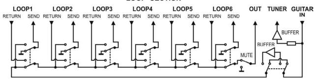
Guitar signal, thru very high impedance (>10  $M\Omega$ ) tuner buffer, is transmitted to TUNER output. It enables using of the tuner during playing.
