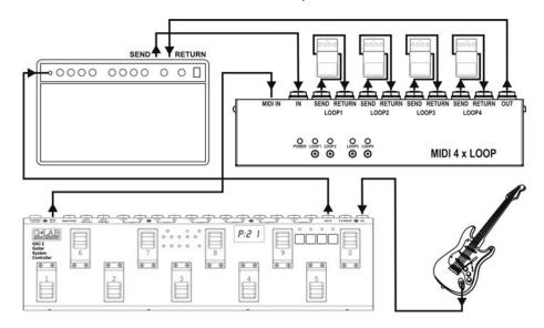
When the GSC is connected to amp FX LOOP the M4L enables to control the effects placed "in front of" (between guitar and amp input).
