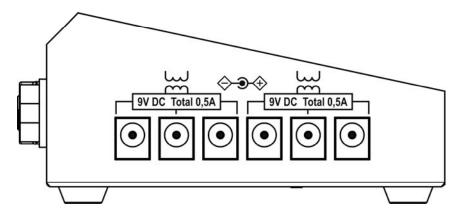
Controller has six 9V DC outputs for supplying the effects in two fully separated sections (500mA each). Before plugging the power supply the pin polarization coincidence should be checked.
