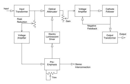
Figure 89. LA-2A signal flow
