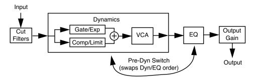
Figure 118. Simplified signal flow within UAD Neve 88RS
