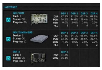
UAD DSP and memory resources used for each installed device, and the ability to enable/disable individual devices, is displayed in the System Information window.
