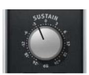
Sustain enables amplification or attenuation of the sustain of a signal by up to  $\pm 24$  dB.
