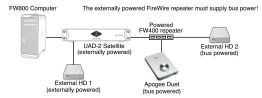
Figure 43. Proper connection of bus powered FireWire devices
