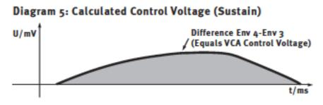
Figure 169. SPL Transient Designer Sustain Control Voltage
