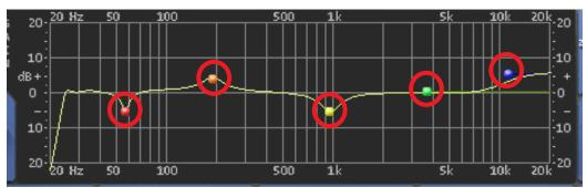
Figure 47. The Curve Control Bats can be used to control EQ band frequency, gain, and Q
