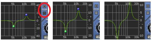
Figure 46. Vertical resolution of the Response Curve can be changed with the Zoom buttons
