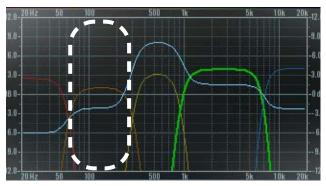
A band can also be selected by clicking within the area of the band in the EQ Display. For example, clicking within the area shown here will select the LMF band.
