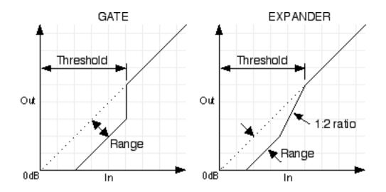
Figure 119. The Neve 88RS Gate/Expander diagram
