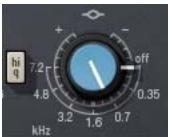
The midrange band is controlled by dual-concentric knobs, delivering smooth semi-parametric midrange equalization with a choice of two bandwidths. The inner knob controls the band gain, and the outer ring selects the frequency or band disable.
