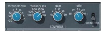
Controls in this section only function when the compressor is enabled with the "compress In" switch (the Power switch must also be on).
