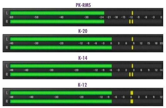
Figure 139. Precision Limiter Meter Types
