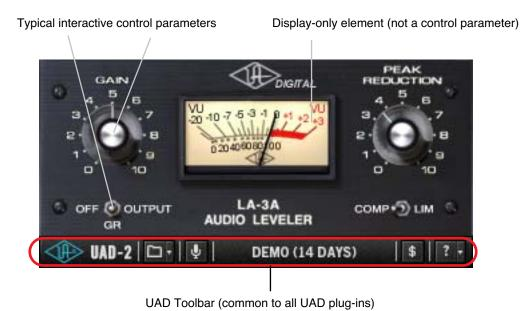
Figure 18. A typical UAD plug-in window
