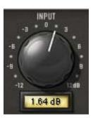
The Input Level knob controls the signal level that is input to the plug-in. Increasing the input will generally result in more processing (depending on the settings of the other parameters).
