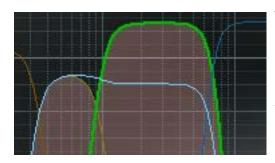
When a band is in Solo mode, its curve in the EQ Display is highlighted.
