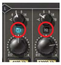
Each band can be individually engaged with the Enable button. All bands default to disabled. When a band is enabled, the button glows blue. To enable a band, click the Enable button or move the band Gain knob.
