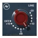
The Input Gain control sets the level at the input of the plug-in. The range is from -20 dB to +10 dB.
