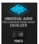
The Power Switch determines whether the plug-in is active. This is useful for comparing the processed settings to the original signal, or to bypass the plug-in to reduce the UAD DSP load (load is not reduced if "UAD-2 DSP LoadLock" on page 73 is enabled).
