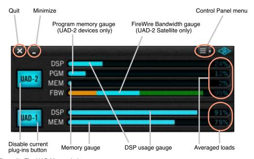
Figure 7. The UAD Meter window
