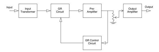
Figure 91. 1176LN signal flow
