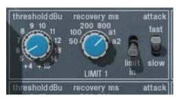
Controls in this section only function when the limiter is enabled with the "limit In" switch (the Power switch must also be on).
