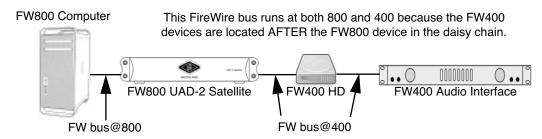
Figure 39. FireWire 800 bus – devices running at 800 and 400 megabits (recommended setup)
