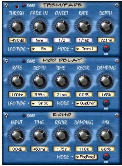
Figure 129. The TremModEcho plug-in contains three modules
