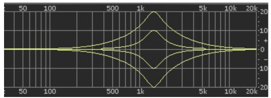
Figure 49. Parametric Type I response
