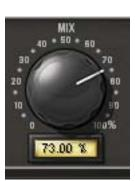
The Mix knob is a mix control for the plug-in. Mix determines the balance between the original and the processed signal.
