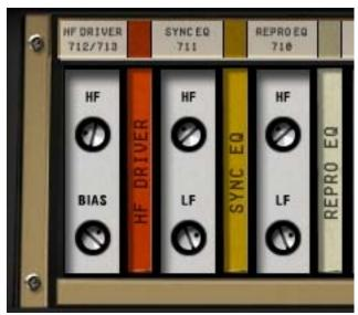
Figure 175. The calibration controls for Studer A800
