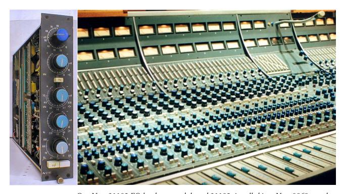
One Neve 31102 EQ hardware module and 31102s installed in a Neve 8068 console
