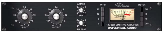
Figure 92. The 1176LN plug-in window
