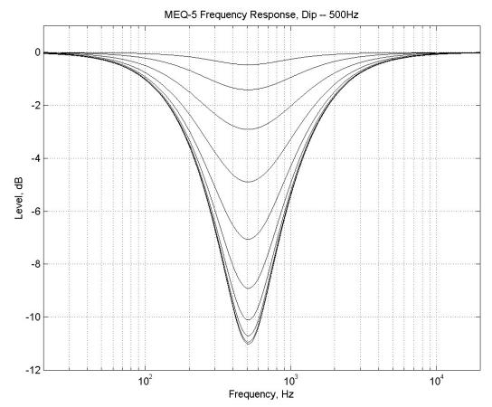
Figure 149. Pultec MEQ-5 Dip Response
