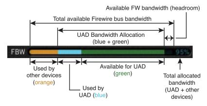
Figure 41. Elements of the UAD FireWire Gauge
