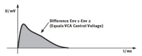
Figure 166. SPL Transient Designer Attack Control Voltage
