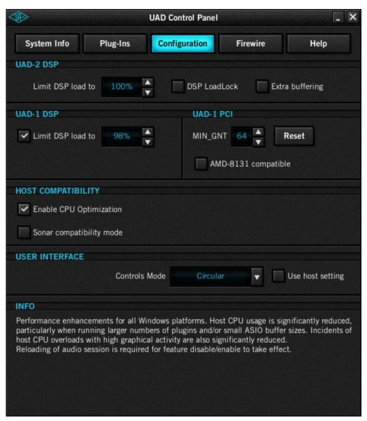
Figure 12. The UAD Configuration panel
