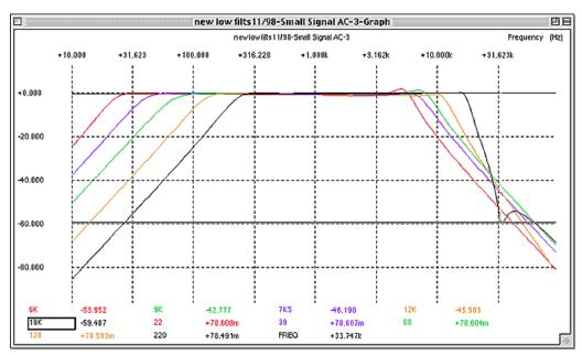
Figure 104. High Pass and Low Pass filter response curves (standard version)
