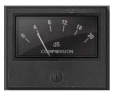
The Gain Reduction VU-style meter displays the amount of gain reduction occurring in the compressor. Higher values indicate more gain reduction.
