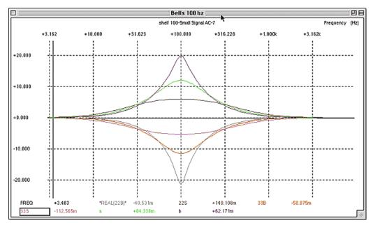
Figure 102. Effect of Bandwidth control on response curve in Bell mode
