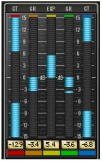
Realtime display of Precision Multiband dynamics processing is shown in the Dynamics Meters. This area also contains the band enable and band solo controls.
