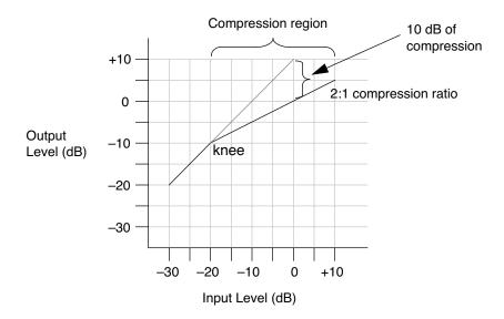
Figure 88. Input and output curve of compressor with 2:1 ratio and -20 dB threshold
