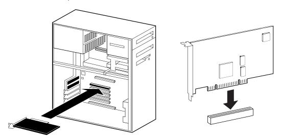
Figure 2. UAD-1 card installation in PCI slot. UAD-2 in PCIe is similar.
