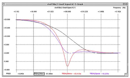
Figure 103. Effect of Bandwidth control on response curve in Shelf mode
