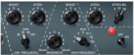
Figure 145. Control grouping within the Pultec EQP-1A
