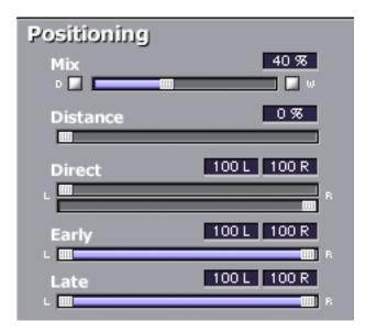
Figure 157. RealVerb Pro Positioning panel
