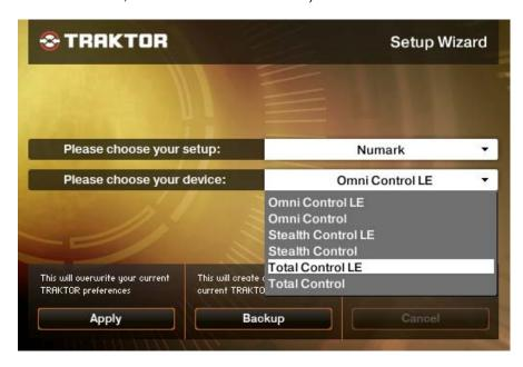
Your Total Control USB MIDI controller is now configured to control Traktor LE! If you are using the Numark DJ|iO as your computer audio interface, proceed with the steps below to configure it with Traktor LE.
