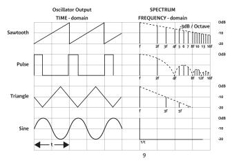
the signal is actually generated as a sequence of calculated numbers. (Conventionally, these are generated at the standard sampling rate for music CDs, 44.1KHz.) This does not become motion until, at the output of the synthesizer, the number stream is converted to variations in voltage, and then amplified, and then used to drive a loudspeaker. (A loudspeaker is a motor that moves back and forth instead of around and around.)
