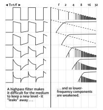
Any device or mechanism that passes along faster motions better than slower ones is a highpass filter.
