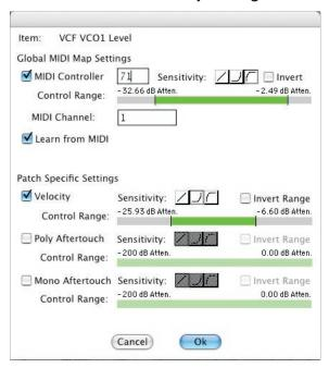
Select the *controller number*, either by directly typing it in, or by twiddling the physical control on the MIDI device you intend to use.
