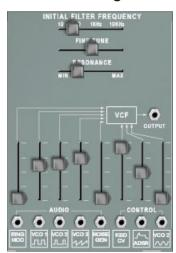
The *Voltage Controlled Filter* has variable cutoff frequency (Fc) and resonance (Q). The response below Fc is flat down to DC; above Fc the response falls off at 24Db per octave. Fc range is from 10Hz to 10KHz without control voltages; under voltage control, Fc can be driven as far down as 1 Hz and as high as 20KHz.
