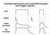
A device whose output is intended to control some time-varying attribute of an event is called an *envelope generator*. These are sometimes referred to as transient generators, to call attention to the fact that their output is not constant but transient.
