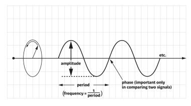
Picture a point on that rotating circle, leaving a trail behind as it rotates, like an airplane propeller. Picture the trail, stretched out behind like a coil spring, and ask yourself:
