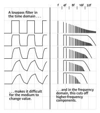
Any device or mechanism that passes along slower motions better than faster ones can act as a lowpass filter.
