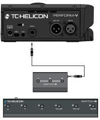
Connecting a Switch-3 or Switch-6 to your Perform-V's pedal input
