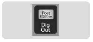
being sent to the FireWire bus is pre-Fat Channel. The Dig Out button is only optional when one of the 16 inputs is selected. The Subgroups, Main Output, Aux bus, Aux Ins and Internal Effects Returns automatically send their signals post Fat Channel dynamics and EQ. All FireWire sends are pre-fader except for the Subgroups and the Main Outputs. For more information on using your StudioLive as an audio interface, please consult Section 3.
