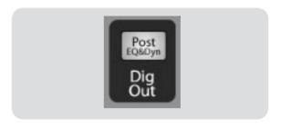
the signal sent via FireWire will be post-trim and post analog insert (if applicable). As previously discussed in Section 2.3.4, the Dig Out button is not operable for the Subgroups, Main Outputs, Aux bus, Internal FX Returns, and Aux Inputs. The Subgroups, Main Outputs, and Aux Inputs are also sent post-fader to their FireWire sends.
