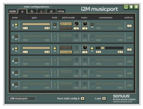
Figure 5: MIDI Configuration / Zones. The currently active MIDI Configuration is highlighted so you know if the one you are editing is currently active or not
