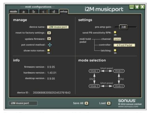
Figure 6: The setup tab lets you change global settings, manage your device and gives information on the version of hardware and firmware in your i2Mmusicport.
