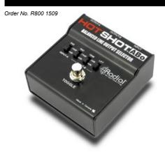
The Hot Shot ABo is a balanced line selecting device that toggles a signal between two destinations. It features 100% passive operation with latching footswitch and therefore does not require any type of powering whatsoever. To add versatility both outputs are equipped with a -15dB pad and output B is equipped with a secondary -6dB trim to reduce the output going to a more sensitive source.
