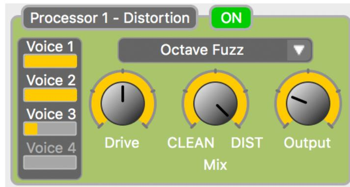
Adds distortion to any of the four Voices. Distortion is a very commonly used in analog modular synthesizers - it not only adds intensity to the sound, its high harmonic content heavily accentuates the sound of the modulating filters. The C4 includes 13 types of distortion, anything from a subtle drive effect to extremely fuzzy Foldback effects.
