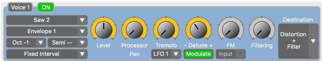
The C4 features four individual Voices. Assign each Voice to any one of the possible options: Sine, Square, or Saw Wave Oscillator, Monophonic Pitch Shifter, Polyphonic Pitch Shifter, or the dry signal routed directly to the envelope filters and/or distortion block. Mix together any combination with each Voice's dedicated Level and Pan Controls. All four Voice modules feature the same control set.
