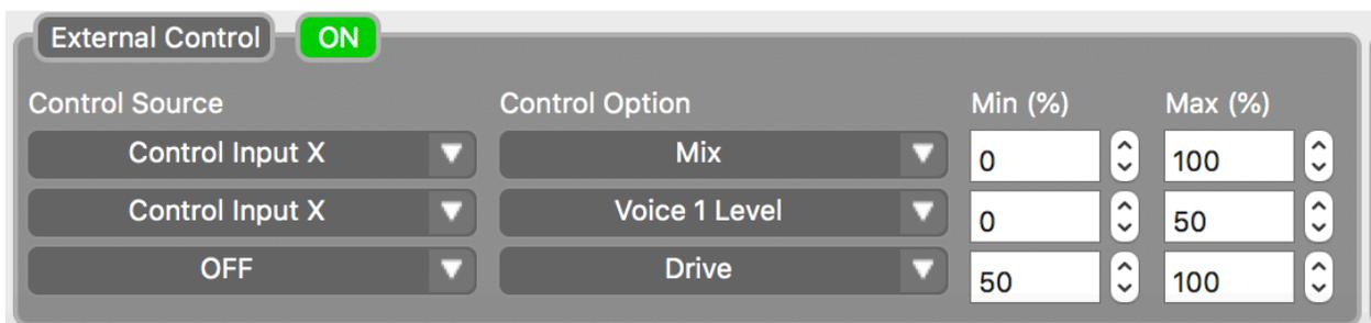
The External Control block is where external expression control is assigned to devices like the Source Audio Dual Expression Pedal, Hot Hand 3 Wireless Controller, and expression devices connected to a Neuro Hub. All external control expression devices connect to the CONTROL INPUT jack on the topside of the pedal with a 1/8” TRRS cable.
