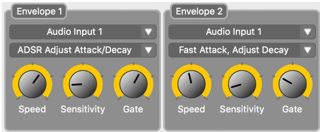
The Envelopes control amplitude and filter modulation of the each C4 Voice. Both Envelopes 1 and 2 run independently of each other and each can be assigned a different set of Voices.
