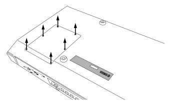
**ENOTE** Keep the removed (6) screws in a safe place. They will be used when attaching the Plug-in board cover to the keyboard again.
