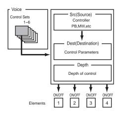
The Element Switches (Page 70) will be disabled if the Dest parameter setting is not specific for Elements (i.e., for settings 00 to 33). By creating Control Sets, you can change sounds in a variety of ways.
