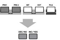
• Press the MEMORY [PRE2] key while holding down the MEMORY [PRE1] key (or vice versa) to select the Preset (PRE) Memory of the Drum Voice. Then use the [DATA] knob to select the Drum Voice.
