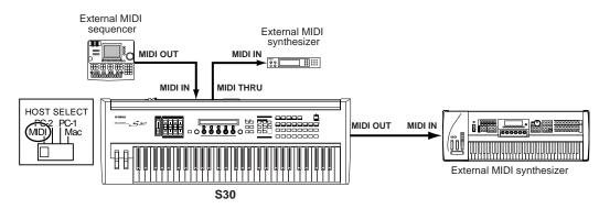
With the above MIDI connections, you can send MIDI data from the MIDI OUT connector while MIDI data from the external sequencer can be sent to an external MIDI synthesizer via the MIDI THRU jack.
