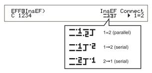
□ Settings: 1 = 2 (parallel),  $1 \rightarrow 2$  (Insertion Effect 1 to 2),  $2 \rightarrow 1$  (Insertion Effect 2 to 1)
