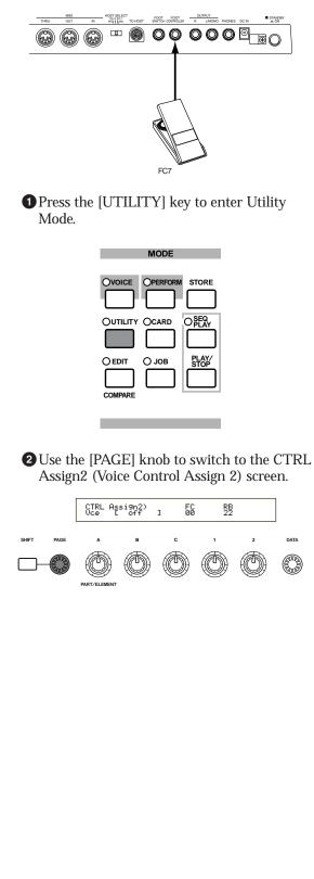
**3** Use Knob [C] to select "01:ModWheel" (Modulation Wheel).
