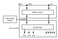
The controllers can also send MIDI Control Change messages to control the parameters of external MIDI devices. These assignments are found in the VOICE (Vce) CTRL Assign1/2 screen of Utility Mode.
