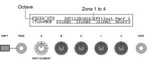
Use Knob [B]/[C]/[1]/[2] while holding down the [SHIFT] key to select the MIDI Transmit Channel (1 to 16).
