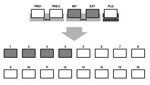
• Press the MEMORY [EXT] key while holding down the MEMORY [INT] key (or vice versa) to select the Internal/External (INT/EXT) Memory of the User Drum Voice. Then use the [INC/YES] or [DEC/NO] keys to select the Drum Voice.
