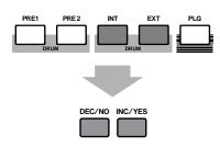
• Press the MEMORY [EXT] key while holding down the MEMORY [INT] key (or vice versa) to select the Internal/External (INT/EXT) Memory of the User Drum Voice. Then use the [DATA] knob to select the User Drum Voice.
