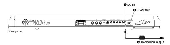
• Make sure that the instrument's STANDBY/ON switch is at the STANDBY(off) position.
