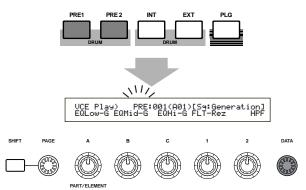
Once you have selected one Drum Voice, you can easily switch to another by simply using PROGRAM keys [1] to [8], the [INC/YES] and [DEC/NO] keys or the [DATA] knob.
