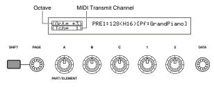
This lets you set the MIDI Transmit Channel by turning Knob [A] and holding down the [SHIFT] key. The settings for Voice Play Mode are transmitted on this MIDI channel.
