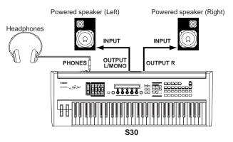
When using just one powered speaker, connect it to the OUTPUT L/MONO jack on the rear panel.
