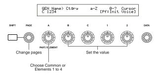
While holding down the [SHIFT] key, you can use Knobs [A], [B], [C], [1] or [2] to move the cursor to the respective parameter without changing it's value. You can also move the cursor using the [DATA] knob or the [INC/YES] and [DEC/NO] keys while holding down the [SHIFT] key.
