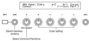
You can use Knobs [A] to [C] and Knob [1]/[2] while holding down the [SHIFT] key to move the cursor to each respective parameter. The cursor can also be moved using the [DATA] knob or the [DEC/NO] and [INC/YES] keys while holding down the [SHIFT] key.
