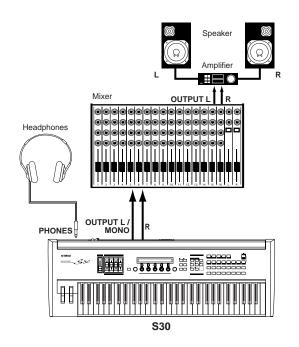
Connecting a pair of headphones does not affect audio output from the OUTPUT (L/MONO and R) jacks. You can monitor the same sounds via headphones and at the OUTPUT jacks.
