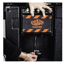
**Bassbock** retainer plate: Align the oval holes in the BASSDOCK retainer plate with the threaded inserts in the cabinet. Replace both thumb-screws, being careful not to cross-thread them. Amp should now be firmly retained with the controls just below the top surface for protection.
