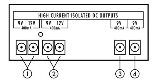
1, 2) 9V and 12V high-current output pairs. Each pair is an isolated output section providing up to 400mA.
