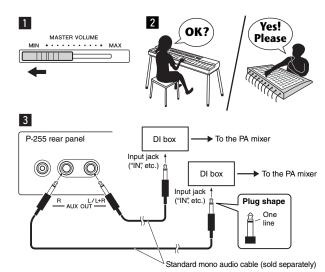
• If only one of the DI box channels is available for use with your digital piano, connect it to the [L/L+R] AUX OUT jack using a standard mono audio cable. In this configuration, your left and right signals will be mixed and output from the instrument in mono.
