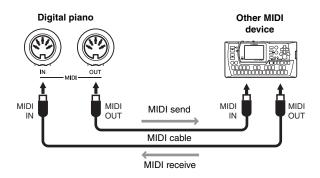
The digital piano's MIDI related settings—such as send channel, receive channel, and the type of data sent and received—can be configured using the corresponding Function parameters (page 40).
