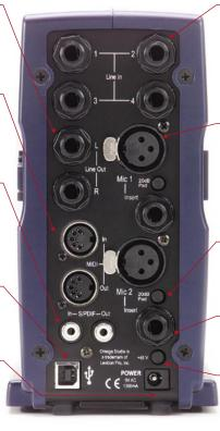
MIC LEVELS: Control the input gain of the professional-grade dbx<sup>®</sup> mic preamps. Up to 50dB of gain!
