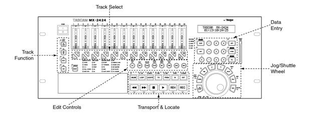
This diagram shows the different control sections of the MX-2424's front panel.
