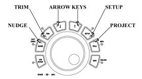
To the right of the Jog/Shuttle Wheel are your MX-2424's two main menu buttons ([SETUP], [PROJ/NEW]. The two buttons directly above the Jog/Shuttle ([Down Arrow] and [Up Arrow]) give you value up and down control. The two buttons to the left of the Jog/Shuttle ([NUDGE/CAPT EVENT], and [TRIM]) are for nudge and trim functions. The Jog/Shuttle Wheel can be used for dialing in numerical values, selecting characters, and scrolling.
