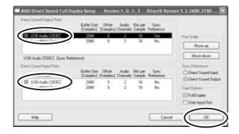
Make sure that "USB Audio CODEC 1/2" are shown in the [Port System Name] field, and check the [Visible] column in the Device Setup window. Click [OK] to close the window.
