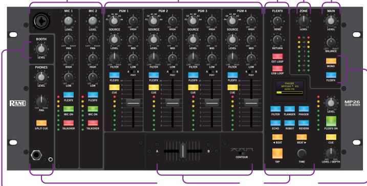
The **Booth** Output includes a Level control and auto-mono balanced 1/4" TRS outputs. **Phones** accept both 1/4" and 3.5 mm plugs. Level, Pan and Split Cue controls support different monitoring styles. The **Crossfader** is a no-noise, no-bleed magnetic fader with three contour settings.
