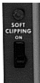
Activation of the overload circuit
