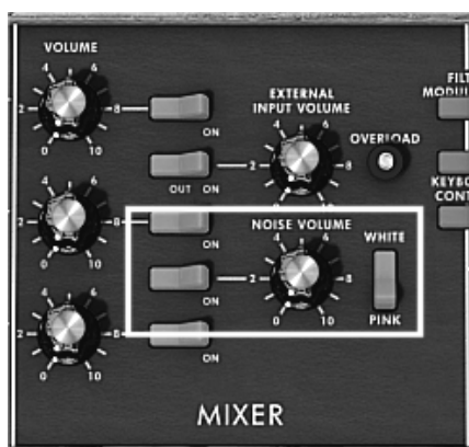
The noise generator set on the mixer
