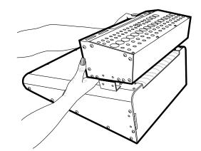
8. Gently press the Pod down until it is flush with the mixer bottom surface. Make certain that none of the wires are pinched, then secure the Pod with the four screws shown below (saved from step 3).
