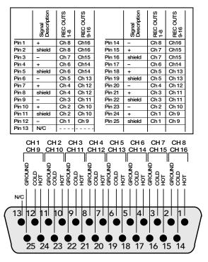
Several companies make DB25-to-DB25 cables specifically for audio, with proper shielding to reduce crosstalk and noise.
