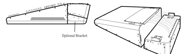
5. Undo the four screws and remove the metal escape hatch (not needed for the rear mounting position). Keep the screws and the plate safe. Make sure that nothing accidentally falls inside the mixer. Pet rodents like nothing better than to nibble on electrical connections and build nests inside, so be warned.
