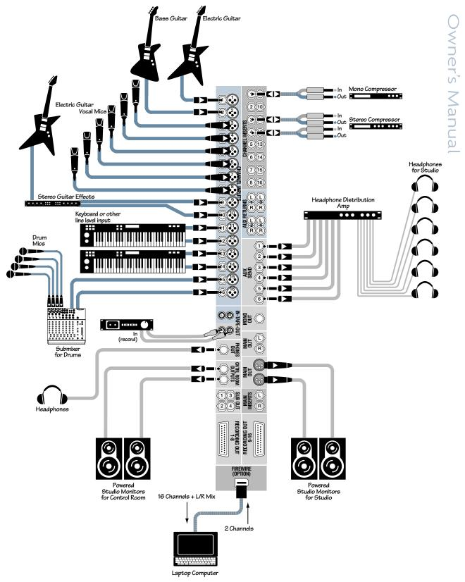
The optional FireWire card provides a digital direct output for each channel, as well as the L/R Mix. Two tracks can be returned to the Onyx from the computer for playback monitoring in the Control Room Outputs, or mixdown to two tracks at the TAPE OUT. The six AUX SENDS provide six separate mono headphone mixes to the talent.
