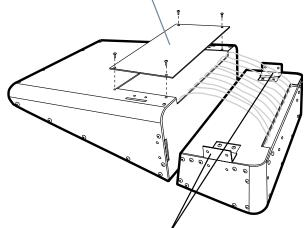
Remove the two L-shaped brackets from the pod section by undoing the two screws on each one. Look at how they come out of the slots as the screws are removed, and then add them to the main section in the same way. Secure the brackets with the same screws.
