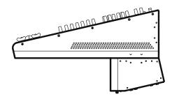
3. Using an optional bracket, it can also be fitted so the connections face the same direction as the console side (the fun side) of the mixer. This will take up 17 rack spaces.
