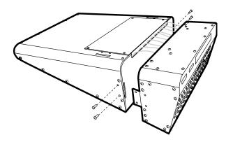
4. **Gently** pull the pod section away from the main section, and rotate it so the connections are face downwards. Do not strain the electrical wires joining the two.
