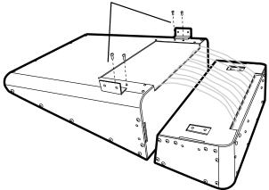
7. Gently pick up the Pod without straining the wires, rotate it so the connections are pointing up, and place it over the brackets. Tuck the excess wire lengths gently inside the main unit. The Pod has two slots which fit over the brackets, so make sure the slots and the brackets line up.
