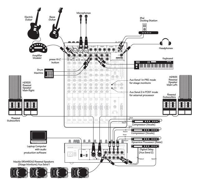
This diagram shows an electric guitar connected to the channel 1 line input via an amplifier modeller, a bass guitar connected directly to channel 2 (hi-z switch in), microphones connected to the channel 3 and 4 mic inputs, a drum machine connected to the channel 5-6 stereo line inputs, and a keyboard connected to the channel 7-8 stereo line inputs. An iPod dock connects to the tape input.
