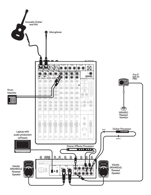
This diagram shows an acoustic guitar mic'd up directly to channel 1 and a microphone connected to channel 2 for vocals. A guitar processor is connected to the insert jack of channel 1.
