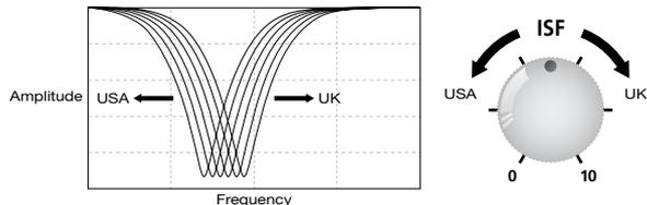
We recommend that to start with the ISF is set to half way and the Tone control set to taste. Then try gradually adjusting the ISF CW and CCW until you find the sound you prefer.
