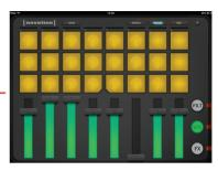
**Volume:** each colum of 8 pads turns into a volume fader. press the pad on row B to reset volume
