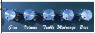
GAIN This controls the level of the preamp and acts quite differently than the dirty channel. Turning this control up will add gain, compression, and some slight break up. To get the cleanest signal possible turn the volume to 8 and use the gain knob for loudness.
