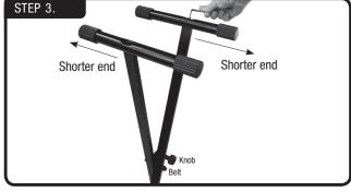
Attach the shorter support arms to the top of the stand. Again, the shorter end of the support arm should be facing out away from the attaching cross-bar center joint (see picture).
