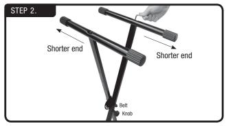
Using the provided Allen wrench and screws, attach the long supports legs to the bottom of the stand. The shorter end of each support leg should be facing away from the attaching cross-bar center joint (see picture).
