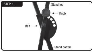
Open the cross-bars until they snap into a stable position. See picture for upright position reference.
