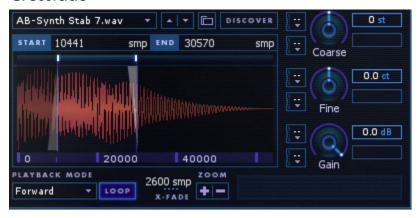
Next to the Loop button is the crossfade value. The crossfade parameter is the number of samples used to blend between the each end of sample selection. Diagonal lines are drawn at the trim points to illustrate what is being used for the cross fades.
