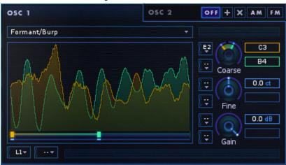
At the heart of the Wavetable Synthesizer Generator are the two wavetable oscillators. Wavetable oscillators are digitally-sampled audio waveforms that can represent simple to complex sounds.
