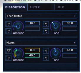
To dirty up your sounds, BreakTweaker's Generators come fortified with an array of distortion effects. Each Generator can host two distortion effects in a serial signal flow. This means that the effect in slot 2 will further distort the signal coming from slot 1.
