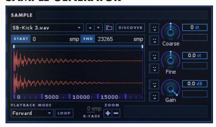
The Sample Generator plays WAV and AIFF audio files. BreakTweaker has a library of audio samples to choose from or you can load your own external samples. The Sample Generator module has control over sample trim points, looping and playback directions, pitch, gain stages, and panning.
