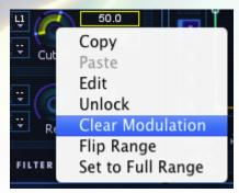
Additional commands to manipulate the modulation knobs and sliders are accessible via the contextual menu. To access the contextual menu right-click on a modulation knob or slider. A pop-up menu will appear with various options. The last three in the menu will manipulate the applied modulation:
