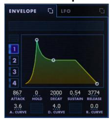
An envelope is triggered by the start of a sequencer note and is used to describe the contour of a sound. This shape is broken into a number of parameters that describe how a sound changes over time. BreakTweaker's envelopes have five parameters: Attack, Hold, Decay, Sustain, and Release. An envelope is triggered by the start of
