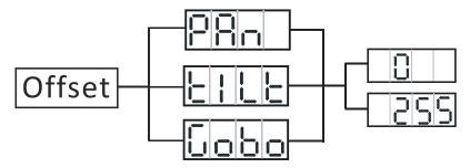
To enter the offset adjustment submenu, press the ENTER button for at least 5 seconds. In this submenu you are able to adjust the pan and tilt home positions and gobo wheel home position.
