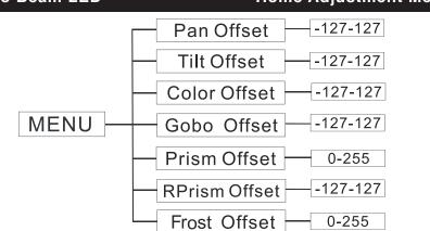
To enter the home adjustment submenu, press the ENTER button for at least 5 seconds. In this submenu you are able to adjust the original position (home position) of certain functions.
