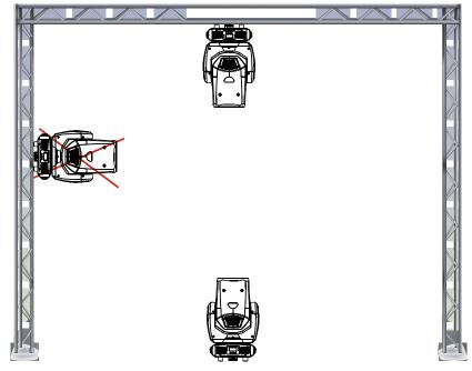
The Inno Beam LED is fully operational in two different mounting positions, hanging upside-down from a ceiling or set on a flat level surface. To avoid internal damage to the unit, never mount the unit on its side as illustrated above. Be sure this fixture is kept at least 0.5m away from any flammable materials (decoration etc.). Always use and install the supplied safety cable as a safety measure to prevent accidental damage and/or injury in the event the clamp fails (see next page).
