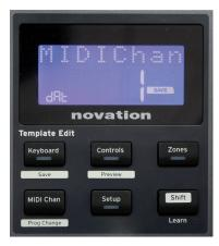
MIDI data can be sent on any one of 16 channels, and will only be received and interpreted correctly if the receiving device is set to the same channel. Press the **MIDI Chan** button to set the channel number.
