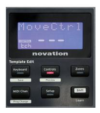
As each template can contain an entire set of configuration settings, make sure you are in the correct template before changing any MIDI parameters. Pressing the **Controls** button 8 enters Control Edit mode, with the display as shown, and the **Controls** button LED lit. Press **Controls** a second time to exit the mode.
