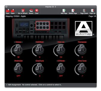
This window will tell you which parameter of the plug-in has been assigned to each encoder by Automap 4, and its current value. Adjusting any encoder will change the value displayed in the window, and you should also be able to see the equivalent control on the plug-in itself varying.
