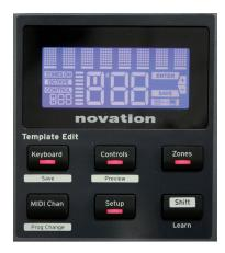
The upper 8-character row of the display shows the Impulse parameter or setting being adjusted. The 3 large characters in the lower row show the parameter value or setting itself. In any of the menus, you can scroll through the available pages with the + and – buttons.
