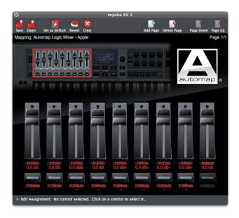
The faders will normally be assigned to Channels 1 to 8, plus Master, and this will be confirmed by the labels below the faders. Higher-numbered channels and additional mixer features (such as Send levels) can be found on additional pages. You can use the **Bank** buttons (**Shift + MIDI**, **Shift + Mixer** by the faders) to scroll 'sideways' and select a further set of eight consecutive channels.
