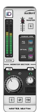
For simple monitoring / listening or in the box mixing it may be cleaner to view just the master section. When fully expanded via ADAT with a device like an ASP800, you can view all channels (after 10 mono slots, a scroll bar appears).
