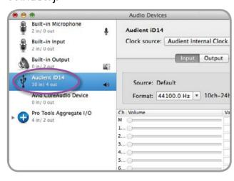
Double check that an appropriate clock source is selected (Internal for master operation), ADAT or S/PDIF clock for external slave operation. Ensure that you see the correct sample rate displayed in the Format drop-down menu.
