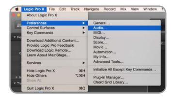
Ensure that iD14 is selected as the active audio device and set the buffer size (to affect system latency). If you are experiencing issues with playback stability and CPU loading, try increasing the buffer size. This appears with "overload" errors and/or pops and clicks and distortion in the audio.
