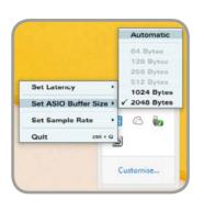
Latency refers to how often iD14 sends and receives its data, for example it is not possible to have a high latency setting and a low buffer size because the buffer would fill up with samples before iD14 has the chance to send them.
