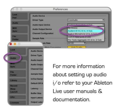
In the Live Audio Preference panel you can set an appropriate buffer size (this can be kept high if you are monitoring input signals for recording via the iD mixer. Ensure that iD14 reports as a 10-in, 4-out device to Live.
