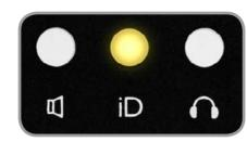
The iD button provides extra functionality in the form of an assignable function button, or it can be used to activate iD14's *ScrollControl* which turns the encoder into a virtual scroll wheel allowing you to control elements of your DAW (see page 22)
