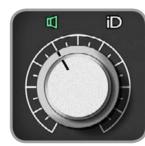
To mute an output, press the encoder quickly. If you only want it to mute momentarily then hold it down, and when it is released it will unmute the audio. In software, press the output icon to mute it.
