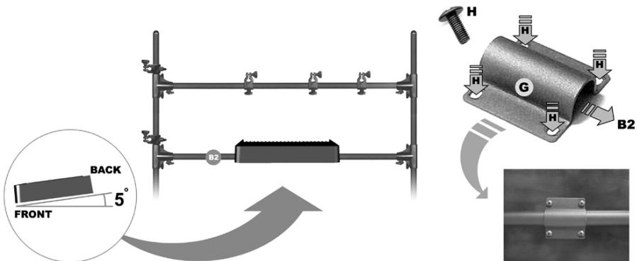
7. Attach the mounting bracket (G) to the back of the iET01 Trigger Box as shown in the figure. Attach to lower horizontal bar as shown in figure and angle accordingly. The iDM01 Drum Machine will rest on top of this.
