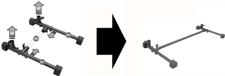
1. Install rubber feet (A1) to the end of each stand base bar (B1). The flat part of the rubber faces the floor. Install one horizontal bar (B2) to the preinstalled horizontal clamp (C) as shown in the picture.
