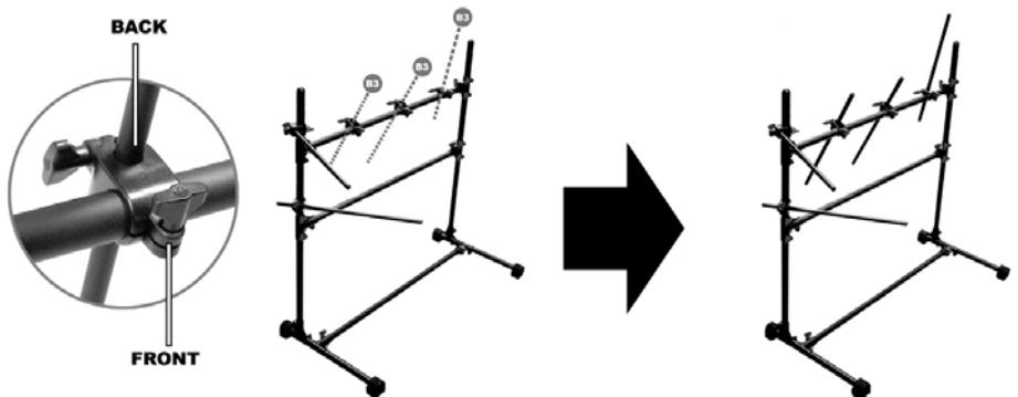
5. Insert three small bars (B3) in the remaining clamps (C) on the top horizontal bar.
