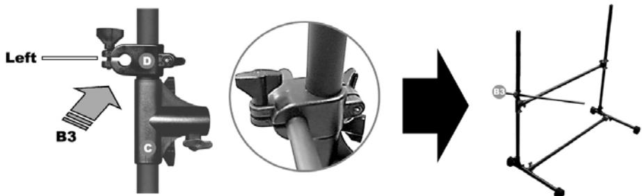
3. Slide one clamp (D) down the left hand vertical bar which will be used for snare-drum pad. Slide one small bar (B3) into the clamp (D) as shown in the figure.
