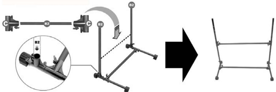
2. Insert two vertical bars (B2) to the remaining slots facing up as shown. Insert two clamps (C) to the ends of one horizontal bar (B2). Slide on the two vertical bars as shown.
