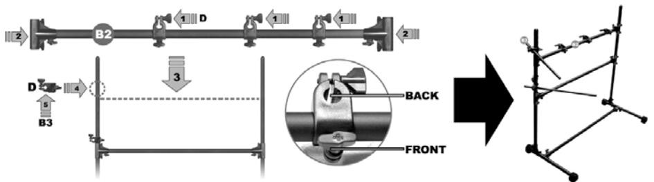
4. Insert three clamps (D) on to a horizontal bar (B2) and put two horizontal clamps (C) on the end. Slide the assembly onto the two vertical bars as shown. Now slide another clamp (D) down the left hand vertical bar which is going to be used for the Hi-Hat. Then slide one small bar (B3) into the clamp (D) as shown.
