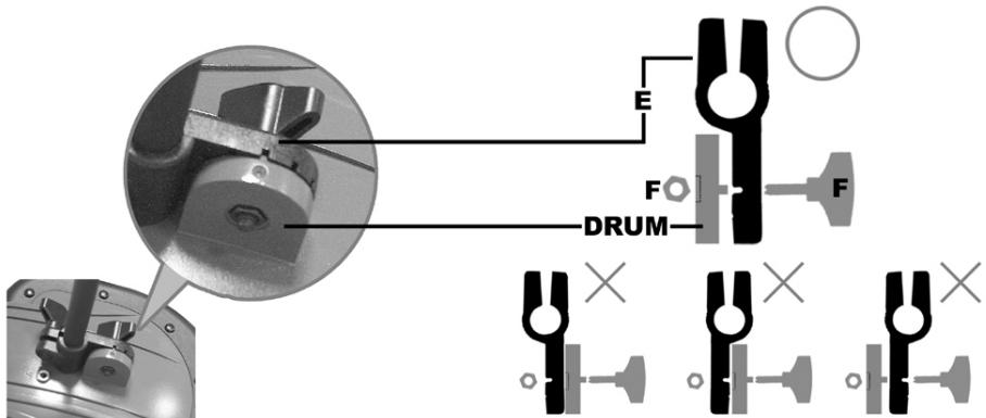
6. Attach five part (A3) to each of the five drum pads. Attach the bolt and nut (F) as shown.
