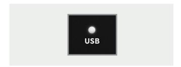
The USB status LED will illuminate as soon as iD14 has achieved stable communication and should remain solidly lit during operation of the unit until power down.
