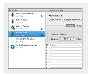
Double check that an appropriate clock source is selected (Internal for master operation), ADAT or S/PDIF clock for external slave operation. Ensure that you see the correct sample rate displayed in the Format drop-down menu.
