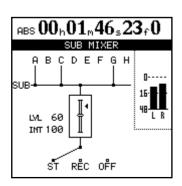
This shows the current assignment of inputs to the sub mixer, and the current assignment of the sub mixer output.
