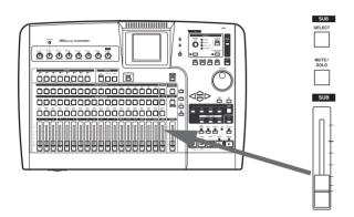
The 2488neo sub mixer facility allows you to add up to eight more inputs (usually on mixdown) to the twenty-four tracks already recorded. These could be inputs from a multi-timbral MIDI device, synchronized using MIDI clock information from the 2488neo driving a sequencer. The eight inputs from A through H are pressed into service here and they feed a bus that can be routed to the stereo bus (or to the recorder in bounce mix—see "Making a bounce mix" on page 58).
