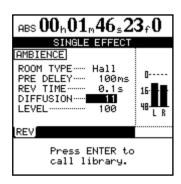
Press the **YES/ENTER** key to enter the library screen to recall a preset effect or a user effect or to save the current parameters.
