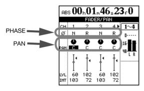
Use this screen to make pan, phase and fader setting for four channels at a time on this screen (linked channels still count as two channels here).
