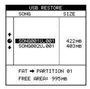
At the bottom of the screen, the restore source partition (FAT), and the restore destination partition (TASCAM partition), and the amounts of unused space on the destination partition are shown.
