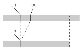
The source and destination are the same, and after the operation, the material which followed the OUT point now moved to follow the IN point. Material which was between the IN and OUT points is deleted. The result is therefore shorter than the original.
