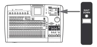
Press the YES/ENTER key. The HD indicator (orange) flashes as data is written to the hard disk (the display also shows this process).
