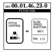
2 If the PITCH CONTROL section at the left of the screen is not active (it is not surrounded by the thicker frame), press the ◀ key to move the cursor there.
