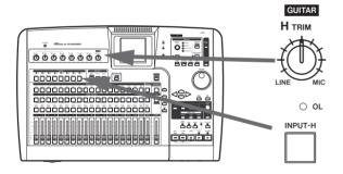
3 Press and hold the INPUT-H key so that it starts to flash. While holding it down, press the SELECT key of channel 1. Now both these keys will flash.
