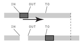
After the operation, the selected section of the source between the IN and OUT points is replaced by silence.
