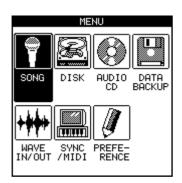
Turn the JOG/DATA dial until the DISK item is highlighted, and then press the YES/ENTER key. The DISK menu appears.
