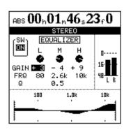
3 Use the cursor keys and dial to select and adjust the EQ parameters for the stereo bus. See "EQ" on page 31 for information about setting methods, etc.
