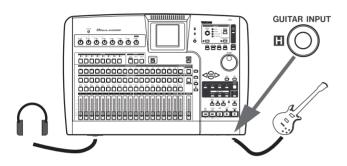
2 Play the guitar, and adjust the level using TRIM control H so that when you play a loud note, the OL indicator above the INPUT-H key lights very briefly. Then turn the TRIM counterclockwise a little to set the appropriate level.
