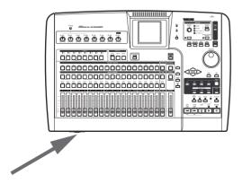
Plug in and turn on the 2488neo. The power switch is on the rear, by the power cord.
