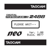
After about 20 seconds, the 2488neo will be ready and the **HD** (hard disk) indicator stops flashing. Adjust the display so that it is comfortable for you to read, using the contrast control.
