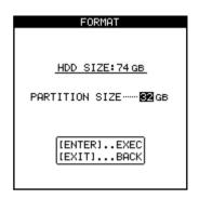
The hard disk size is shown at the top of the screen, and the partition size is shown below this.
