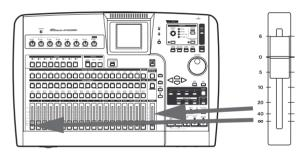
6 Confirm that the MONITOR SOURCE is set to STEREO, and use the MONITOR LEVEL knob to adjust the monitor level. You can also monitor in mono (see "Monitoring" on page 36).
