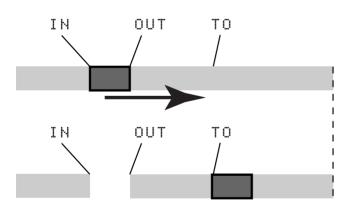
After the operation, the selected section of the source between the IN and OUT points is replaced by silence.
