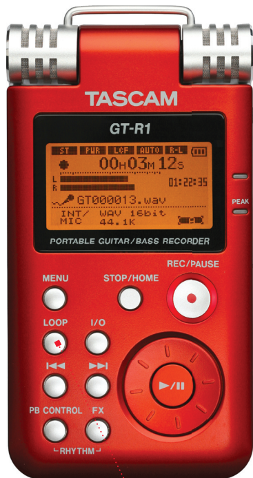
The loop function lets you repeat a specified section of a prerecorded song.
