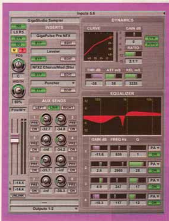
FIG. 4: Changing a channel strip to Wide View mode reveals a full set of dynamics and EQ controls with graphic displays.
