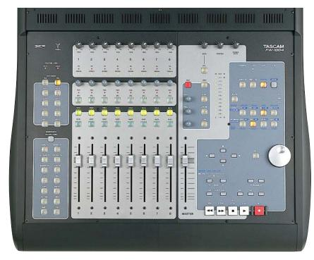
motorized touch-sensitive channel faders, one master fader, and controls for pan, solo, mute and select functions on each channel. Tactile control for four bands of parametric EQ, a jog wheel and a variety of shortcut keys for various popular software applications are also included.
