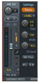
**Width.** Defines the stereo width. 1.00 equals full stereo, 0.00 mono, - 1.00 swapped channels.
