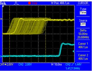
The screenshot shows an extremely jittery SPDIF signal of about 50 ns jitter (top graph, yellow). SteadyClock turns this signal into a clock with less than 2 ns jitter (lower graph, blue). The signal processed by SteadyClock is of course not only used internally, but also used to clock the digital outputs. Therefore the refreshed and jitter-cleaned signal can be used as reference clock without hesitation.
