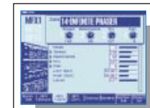
■ MFX Edit Window Use this screen to edit the four major parameters of an MFX processor. Simply twist the Fantom-S/-S88's knobs and the changes are reflected onscreen. More detailed parameter editing is also available.
