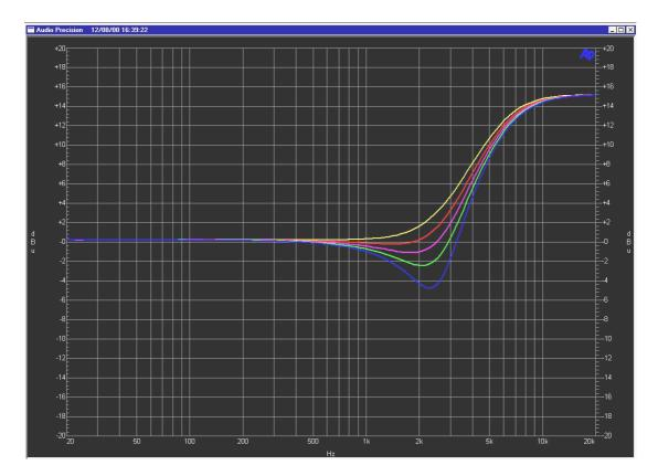
When the HF shelving function is selected, the Q control provides control of the 'overshoot' function.
