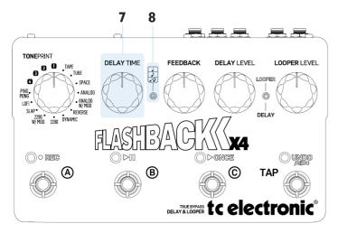
Turn the DELAY TIME knob all the way down for really short repeats. Turn the DELAY TIME knob up until you find your preferred amount of delay time. Turning the DELAY TIME knob all the way up will give you a whopping seven seconds of delay time for most delay types.
