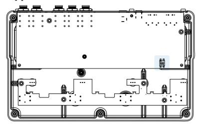
The Flashback X4 Delay & Looper has two bypass modes: **True Bypass** and **Buffered Bypass**. To set the desired mode, you have to open the device.
