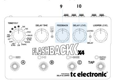
Use the FEEDBACK knob to set the desired numbers of delay repeats. Turning the FEEDBACK knob to the right will give you more delay repeats.
