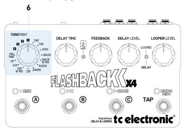
Use the DELAY TYPE SELECTOR to choose the type of delay you want to work with. The Flashback X4 Delay & Looper offers a wide range of delays – from classic tape delays to the pristine sound of a TC 2290.
