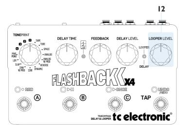
Use the LOOPER LEVEL knob to set the playback volume of the Flashback X4's Looper module.
