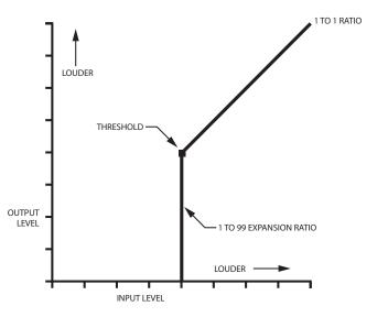
Sounds that are louder than the threshold get "through the gate" unchanged. Sounds that are below the threshold are not heard. Gates can be used to great effect in processing drum tracks where sounds from the other instruments in the drum set leak through the mike of the instrument being recorded. Gates are also used frequently to "gate off" a reverb tail or the ringing from an insufficiently damped drum head.
