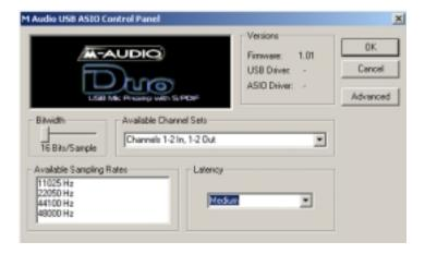
With both stereo pairs enabled, i.e., Channels 1-2 In and Channels 1-2 Out, the Duo behaves as a "2x2" audio device at 16-bits, and at sample rates of 48000Hz and below (that is, 48kHz, 44.1kHz, 22.05 and 11.025kHz). These sampling rate options as well as the bit depth setting will then be available and selectable from within your music program.
