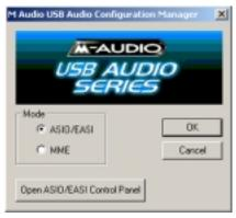
The USB Audio Configuration Manager, when it is first installed, defaults to the "ASIO/EASI" setting. If you are using an ASIO compliant program such as Steinberg's Cubase or Nuendo, or a program that uses "EASI" drivers such as Emagic's Logic, then you should leave the configuration manager set to "ASIO/EASI." The Duo provides its own ASIO and EASI drivers, and the music program you use should be set up to utilize the Duo's ASIO driver (see the section, "ASIO/EASI Operation").
