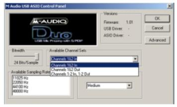
With both stereo pairs enabled at a Bitwidth setting of 24-bits, the Duo will also operate as a 2x2 audio device. In this mode, the Duo is capable of 48kHz or 44.1kHz at either 24- or 16-bits, as set by the music program.
