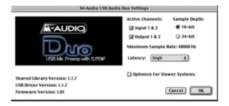
With both stereo pairs enabled, i.e., Input 1&2 and Output 1&2, the Duo behaves as a "2x2" audio device at 16- or 24-bits, and at sample rates of 48kHz and below (that is, 48kHz or 44.1kHz). These two sampling rate options as well as bit depths will be selectable from within your music program.
