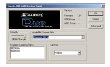
In the M-Audio USB ASIO Driver control panel, to the right of the Bitwidth section, you will see a "Latency" drop-down list that will set the Duo's buffer size. A lower latency setting represents a smaller buffer size, with the lower setting being desirable when using the ASIO drivers.
