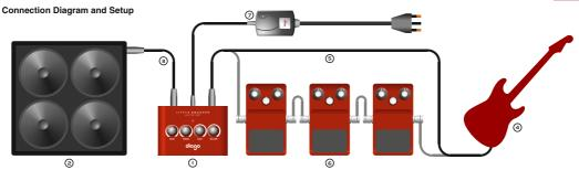
Connect the 1/4" TS JACK SPEAKER OUTPUT of the Little Smasher ① to a passive speaker cabinet ② with an impedance of 4-16 Ohms, using only an adequately rated speaker cable ③. Do not use a signal cable such as a guitar cable, or similar.
