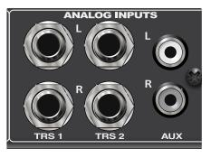
These inputs are for your audio sources (mixer, audio interface, CD player, etc.). Only balanced cables should be used when connecting the balanced TRS inputs of your Central Station to these devices. Because of the Central Station's passive circuitry, using unbalanced cables can reduce the output level and can introduce noise into your system.
