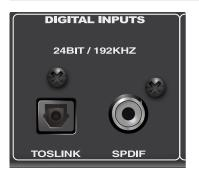
Central Station automatically reads and locks to the sample rate of the incoming digital stream and can receive and lock to sample rates of 44.1, 48, 96, and 192 kHz. Both of these digital inputs are designed for the S/PDIF stereo digital format.
