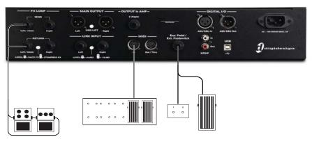
Figure 7. Effects and foot controller connections
