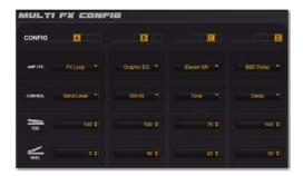
Each of the four Configs can be set to one parameter of one of the devices in the Rig. The Toe and Heel settings govern the top and bottom of the sweep of the control.
