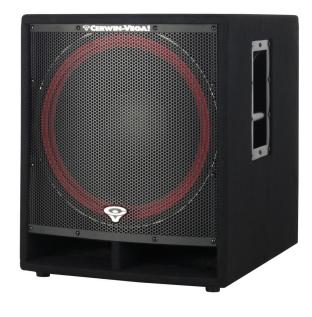
The CVi-118S is a portable, eighteen inch dedicated subwoofer system designed to extend and supplement the low frequency extension of CVi full range systems in live music and playback applications. The CVi-118S features a high power, cast frame eighteen inch transducer with a 3" voice coil for extended use during high SPL applications. Steel handles and pole mount cup are also featured for use as a base for pole mounted full range systems.
